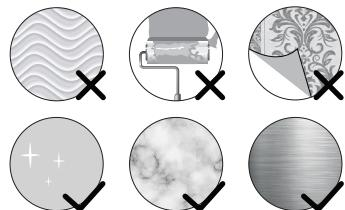
**EN** Transparent adhesive must be mounted on smooth, non-porous surfaces like stainless steel, porcelain, tile, etc. Not for use on textured surfaces such as quartz & stone.
