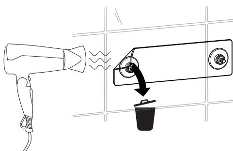
**EN** If you need to remove the installed adhesive, you can use a hair dryer to heat the adhesive surface and slowly separate from mounting surface.
